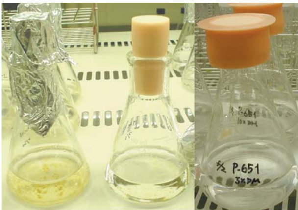
FIGURE 5.2. Erlenmeyer flasks with silicon rubber plugs. Left , covered with aluminum foil; center , a standard silicon rubber plug; right , a silicon rubber plug with an extended shield over the lip of the flask.
