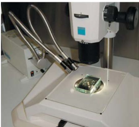
FIGURE 9.8. Isolation of phototactic zooids under observation with a stereomicroscope: Fertile algal tissue is placed at the bottom of a depression slide and the release of zooids is induced by intense illumination from a fiber-optic light source. Released zooids are accumulated at the surface of the medium (lighting from the upper side when they are positively phototactic, and from the lower side when negatively phototactic), and distant from the algal tissue.
