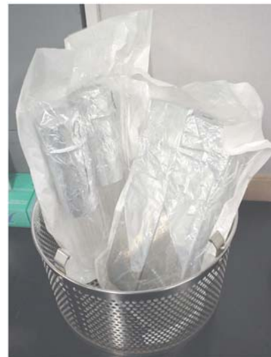
FIGURE 5.9. A stainless steel basket for holding items in an autoclave. The basket contains Pasteur pipette canisters covered with autoclavable bags. Note that the cap junction of a pipette canister is covered by aluminum foil.
