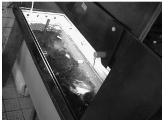
FIGURE 21.8. A 300-liter tank with light-tight PVC hood and slide door in a constant-temperature room. Two halogen lamps on top (not visible) provide culture light. The seawater is aerated by a 20-mm wide PVC pipe on the bottom of the tank with a 2-mm opening at every 10 cm. Note white plastic shields on top of the water carrying marked algal individuals and circulating with the whole biomass within the water column.
