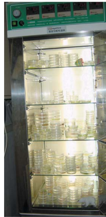
FIGURE 9.3. Temperature-gradient incubation chamber having several closed chambers whose temperatures can be independently controlled.
