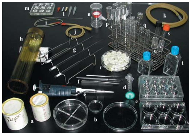
FIGURE 6.1. Assortment of isolation supplies. (a) Screens for removing larger animals and algae; prepared from PVC pipe and Nitex netting. (b) Glass and plastic dishes. (c) Multiwell plates. (d) Syringe with 0.2- \mu\text{m} filter. (e) Pipetteman. (f) Small loop, fine metal probe, and forceps. (g) Pasteur pipettes, with tips drawn to produce micropipettes, arranged on a metal rack. (h) Sterile Pasteur pipettes in plastic can, resting on a simple metal support to keep the opening off the table surface. (i) Glass capillary tube, small tubing, and red mouthpiece. (j) Isolation mouthpiece (red), small tubing connected to final short piece of large tubing that forms a tight seal when a Pasteur pipette is attached. (k) Large isolation tubing with plastic pipette tips at both ends, one serving as a mouthpiece and the other supporting a Pasteur micropipette. (l) Commercial mouthpieces (red, white, yellow) and two plastic pipette tips (right one with pointed tip removed), which can be used as mouthpieces. (m) Glass spot plate that can be used to rinse cells during isolation. (n) Small sterile filter apparatus. (o) Glass slip caps that cover either smooth or threaded test tubes. (p) Smooth, unthreaded test tubes covered with slip caps. (q) Threaded test tubes covered with slip caps. (r) Sterilized test tube caps that can replace slip caps or be used when a culture tube cap is dropped or contaminated. (s) Plastic threaded test tubes (black cap, orange cap), which are sterilized by the manufacturer. (t) Two blue-capped tissue culture flasks, sterilized by the manufacturer.
