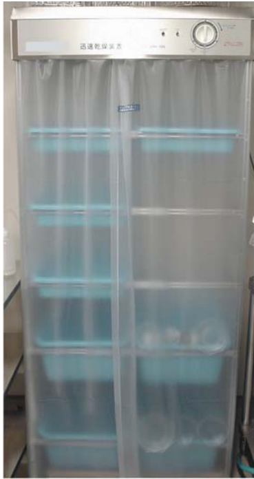
FIGURE 5.1. A dust-proof drying cabinet for storing clean or sterile materials and supplies.
