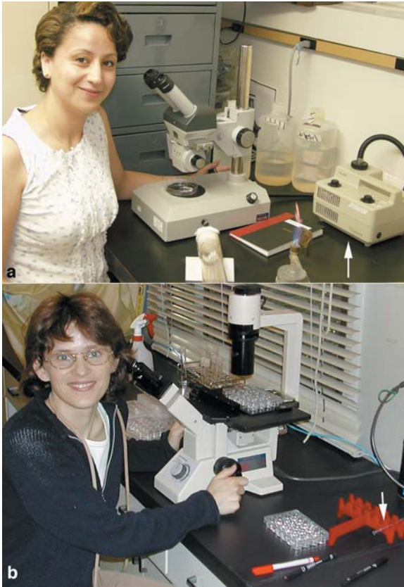
FIGURE 6.2. (a) A Zeiss dissecting microscope (magnification up to 80 \times ), with dark-field illumination delivered by a Schott illuminator ( arrow ; light via fiber optic cable). Dark-field illumination makes tiny cells more obvious than transmitted light. Khadidja Romari. (b) An Olympus inverted microscope (magnification usually up to 400 \times ), with the stage designed for multiwell plates. Note large isolation tube around the neck and the Pasteur pipette that is drawn out and ready ( arrow ). Mary-Helene Noël.
