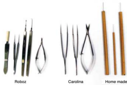
FIGURE 11.3. Dissecting tools. Finest quality and most expensive stainless steel by Roboz, low-cost stainless steel tools from Carolina Biological Supply, homemade needles of wood dowel and sewing needle.
