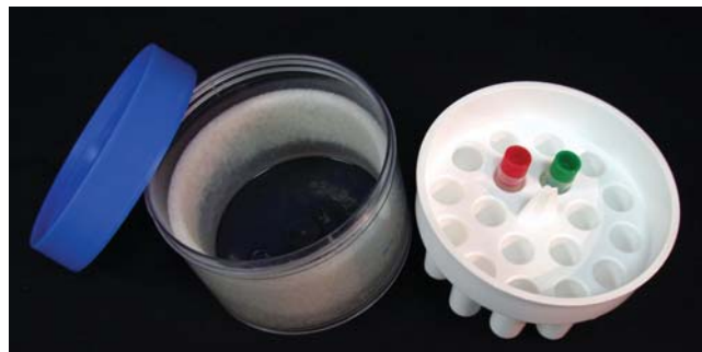
FIGURE 12.3. Mr. Frosty, a passive freezing device. Isopropyl alcohol is placed into the clear plastic container (left). Cryogenic vials (1–2 mL) containing prepared algal cultures are placed into the vial holder (right), the lid is placed securely on the container, and the entire unit is placed into a -80^{\circ}\text{C} freezer (see text for details).
