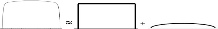
Fig. 7 Left: Typical slip distribution between impenetrable boundaries using the semi-discrete problem formulation. At the boundaries, the slip gradient is singular. Right: Approximation to the actual slip distribution. Singular gradients at the boundaries are approximated by jumps (step functions), so that the approximate slip field consists of slowly varying portion with non-vanishing boundary values
