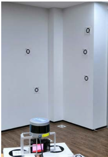
Figure 3. A LiDAR-camera system observing the corners of the wall. Several scenes were collected by changing the pose of the sensor system.
