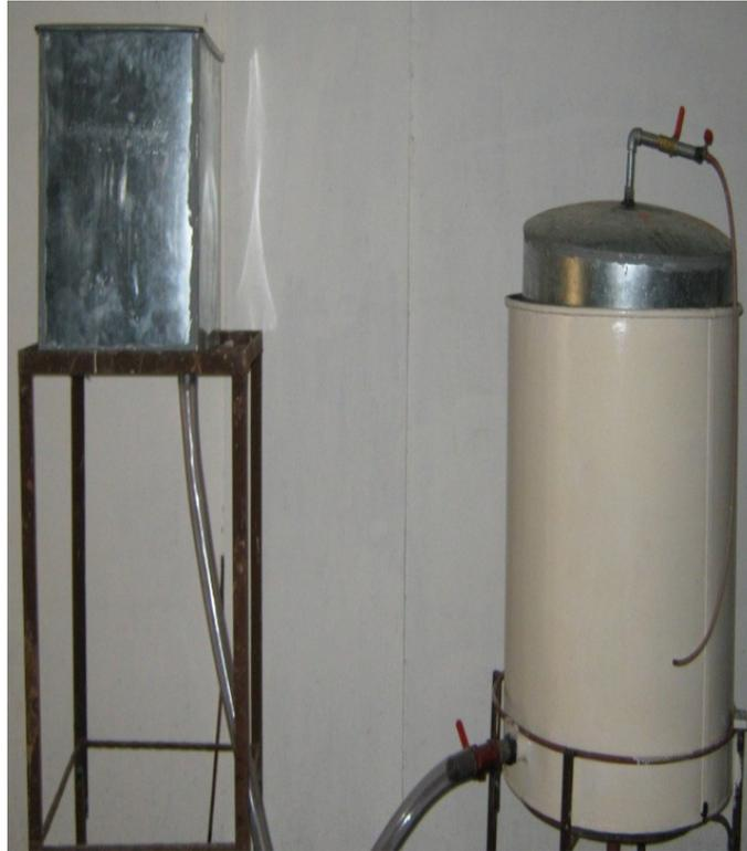
**Figure 3:** Anaerobic digester for generation of Methane Gas from kitchen waste
