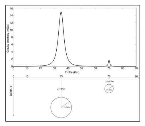
**Figure 1.** The gravity anomaly response due to a model consisting of two buried spheres at subsurface. The parameters used in the computation of the synthetic gravity data are mentioned in the text.
