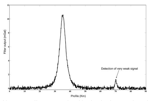
**Figure 4.** Results of the gravity energy filter acting on a weak signal, buried in coloured noise. It can be seen that the detection of very weak signal is also possible when it is immersed in the coloured noise.
