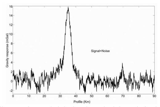
Figure 2. An additive mixture of gravity signal and coloured noise due to two buried spheres at subsurface. The signal due to the shallower spherical body immersed in the coloured noise is obscured and beyond the visual recognition.
