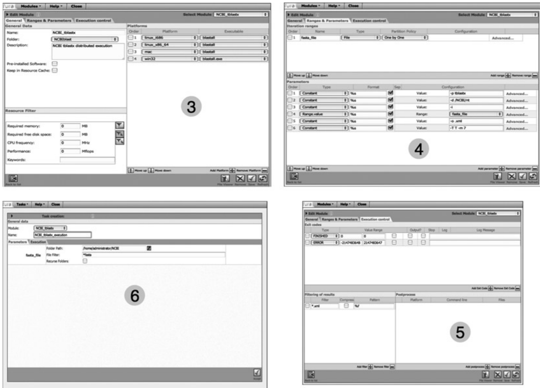
Fig. 3. Key parameters needed to configure a distributed calculation of NCBI Blast using either Fura open source or “Fura In The Cloud” platforms.
