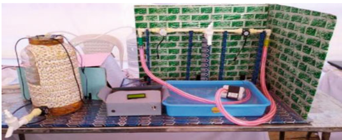
Fig. 8 Smart water governing system
