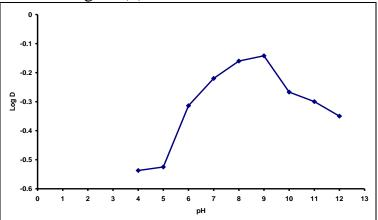
Figure (1): Effect of pH on the extraction of Cd+2 ions
