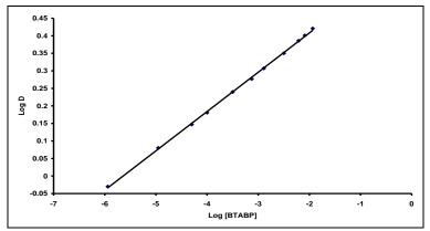
Figure (4): Slope analysis method for extraction Cd+2 ions 3.4.2. Mole Ratio Method
