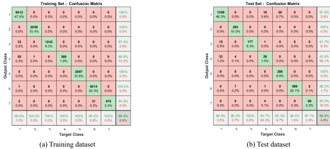
Fig. 14 Confusion matrix for imbalanced full dataset with mean frequency balancing (weight from the full dataset) (Model-C)
