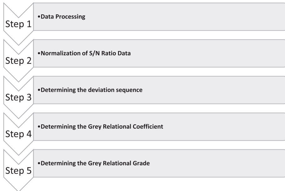
Fig. 5. Multistep sequence used for Grey Relational Analysis.
