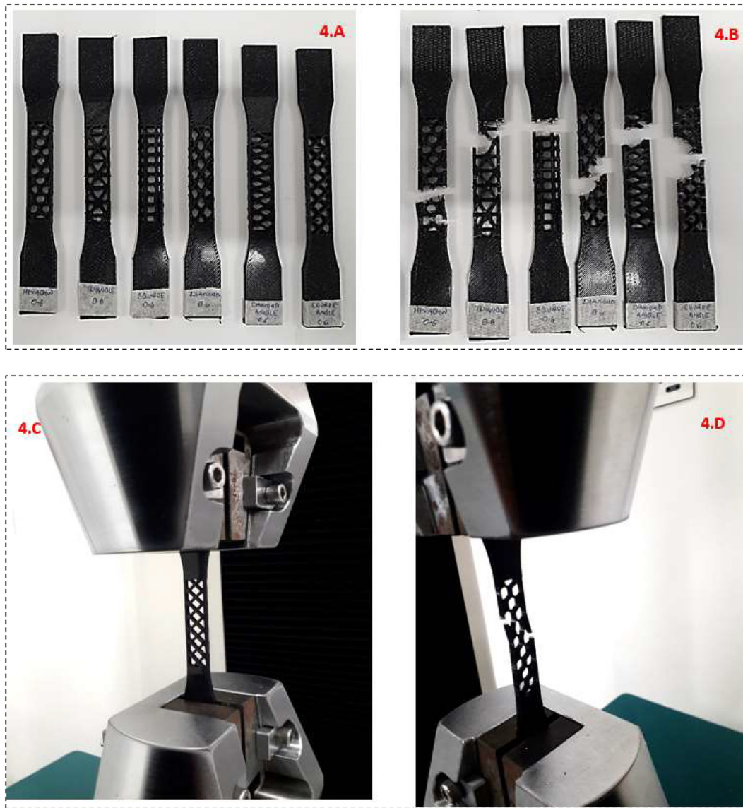
Fig. 4. Patterns used in this study printed at 0.6 mm diameter nozzle as per Taguchi DoE, (A) Patterns before testing (B) Fractured specimens after performing tensile tests (C) Shows the square angle pattern before fracture, (D) Shows the hexagonal pattern after initial fracture took place.
