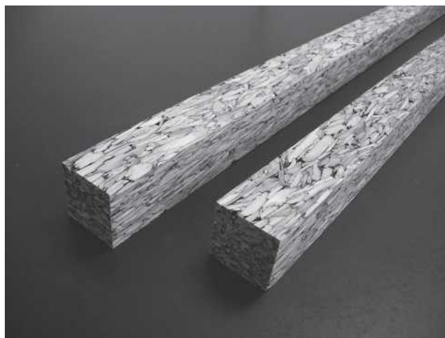
Figure 3. — An example of structural pillars prepared by cutting thick panels of coarse chips. These pillars, used vertically, have a structural function in traditional-type Japanese houses now built according to modern principles.
