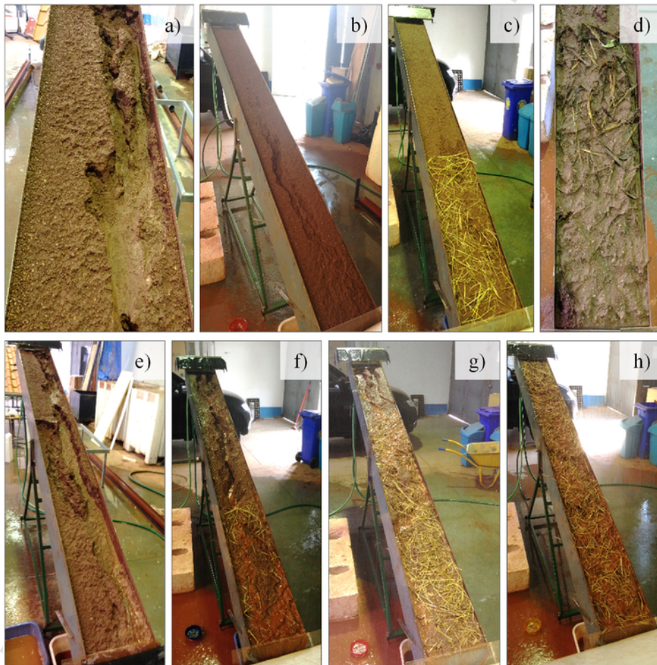
Fig. 6. Photographs of the soil flume: a) Detail of geotextile fabric exposure originated due to extreme erosion; b) Bare soil after W run; c) 1/3-50% after W run; d) Detail of soil deposition on mulch; e) Bare soil at the end of W + F run; f) 1/3-50% at the end of W + F run; g) 2/3-50% at the end of W + F run; and h) 3/3-70% at the end of W + F run. Differences in colour between photographs are related to differences in the photographic camera, luminosity conditions and time at which photos were taken (i.e. during or after an experimental run).
