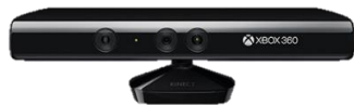
Figure 1: Kinect for Xbox 360 is linked to the PC through an adaptor for the USB port.
