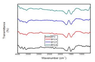
Fig. 2. Fourier Transform Infrared spectra of BPC, BPCH, BPCP and BPCS.
