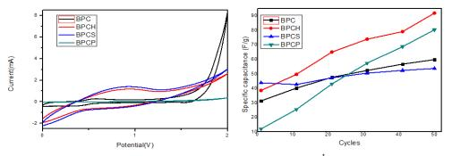
Fig. 3 (a) CV curves of BPC, BPCH, BPCS and BPCP a scan rate of 30 mVs<sup>-1</sup>, (b) Cycle stability of BPC, BPCH, BPCP and BPCS.
