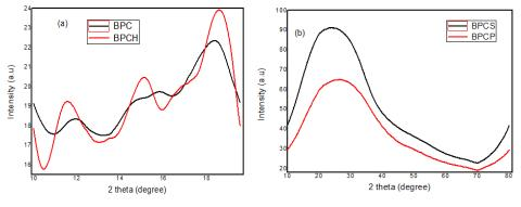
Fig. 1. XRD diffraction patterns of (a) BPC and BPCH (b) BPCS and BPCP.
