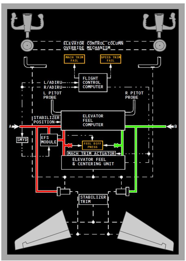
Figure 3 Boeing 737 MAX pitch control system
