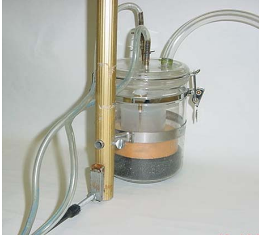
Photograph 1 Special downhole sampling apparatus. The unit is suspended from the extension
