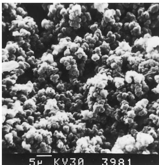
Fig. 1. Scanning electron micrograph of PMMA nanoparticles polymerized by \gamma -irradiation in water. Marker = 500 nm.
