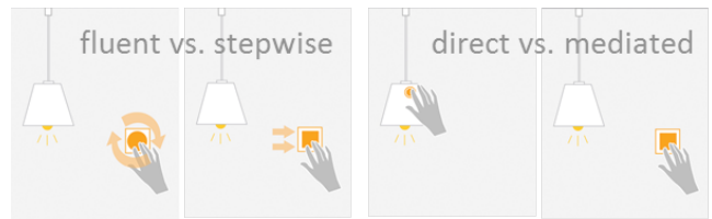
Figure 2. Examples of extracted interaction attributes. Left: Dimmer switch (fluent) vs. flip switch (stepwise). Right: Switch on the lamp (direct) vs. wall switch (mediated).
