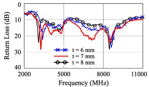
Fig. 7. Measured return loss as a function of the width  $t$  of the wide-ended portion of the radiating arm. Other parameters are the same as given in Fig. 2.
