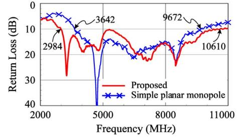
Fig. 2. Measured return loss for the constructed prototype with  $L = 60 \text{ mm}$ ,  $t = 7 \text{ mm}$  and a corresponding simple planar monopole [the antenna in Fig. 1(c)].
