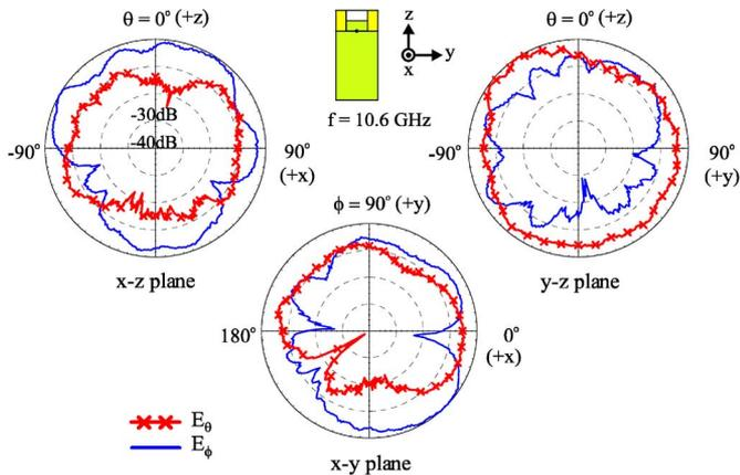
Fig. 5. Measured radiation patterns at 10.6 GHz for the constructed prototype studied in Fig. 2.
