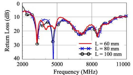
Fig. 8. Measured return loss as a function of the system ground-plane length  $L$ . Other parameters are the same as given in Fig. 2.
