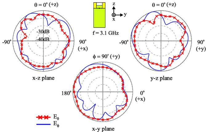
Fig. 3. Measured radiation patterns at 3.1 GHz for the constructed prototype studied in Fig. 2.
