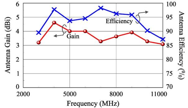
Fig. 6. Measured antenna gain and simulated radiation efficiency versus frequency for the constructed prototype studied in Fig. 2.
