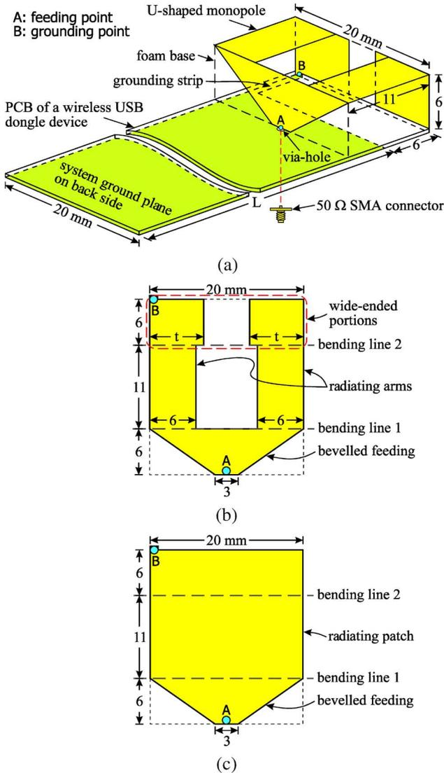
Fig. 1. (a) Configuration of the proposed, internal-UWB monopole antenna mounted on the PCB of a wireless USB dongle. (b) Detailed dimensions of the proposed antenna unbent into a planar structure of a U-shape. (c) Detailed dimensions of a corresponding simple planar monopole unbent into a planar structure.
