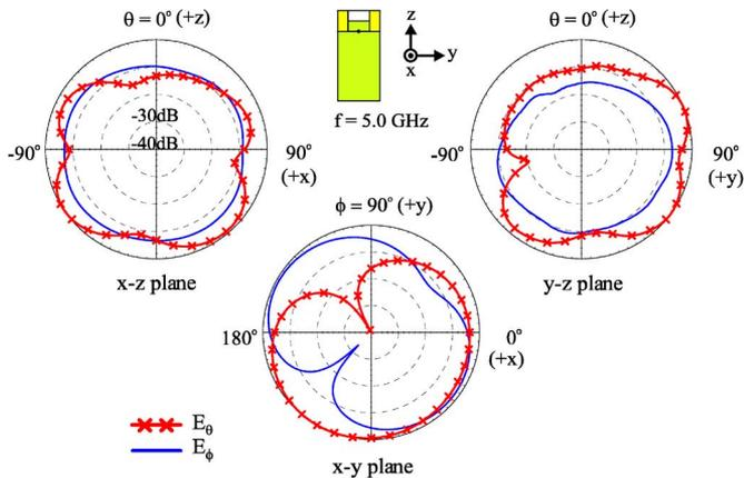
Fig. 4. Measured radiation patterns at 5 GHz for the constructed prototype studied in Fig. 2.
