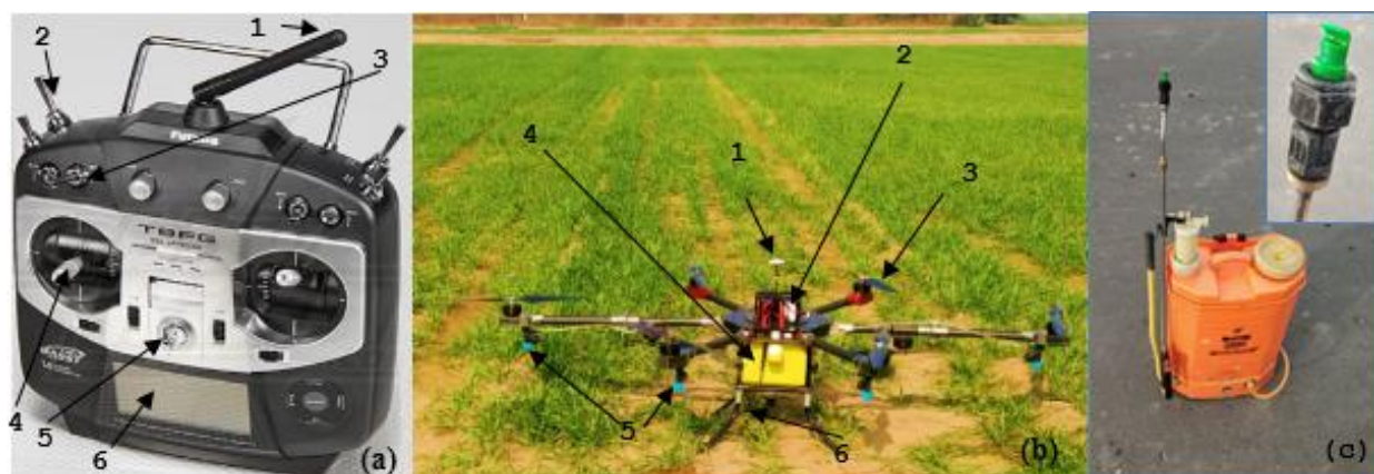
(a) 1. Antennas 2. Sprayer switch 3. RTH Switch 4. Stick 5. Power switch 6. Screen (b) 1. GPS 2. Battery 3. Motor and propeller 4. Sprayer tank 5. Nozzle 6. Pump
