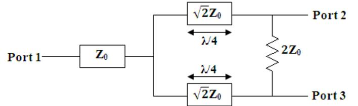
Fig. 1 Transmission line modelling of WPD
