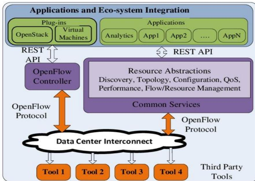
Fig.4. The use of OpenFlow for Cloud and Datacenter
