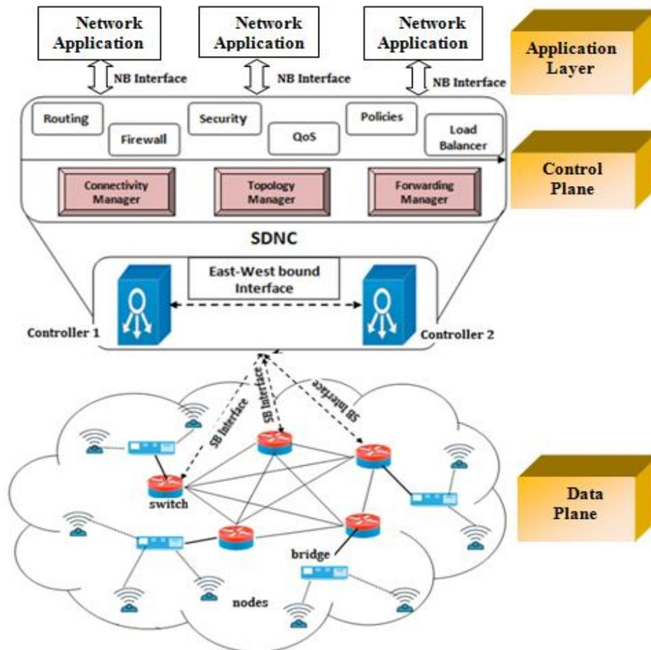
**Fig.3.** SDN architecture for Networks
