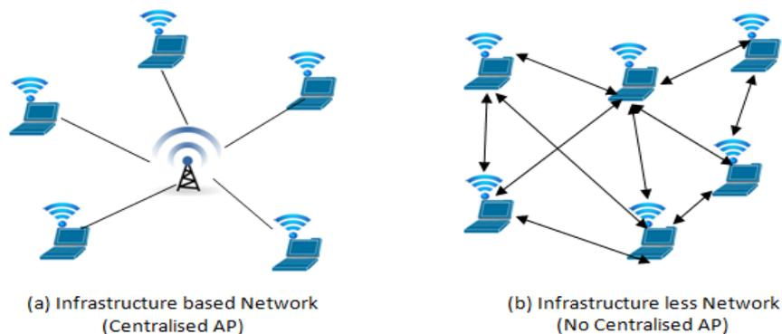
**Fig.1.** Classification of wireless network
