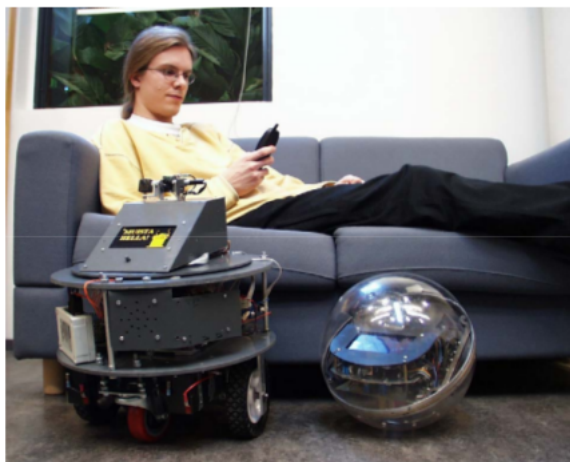
Figure 2.1: Information home robots used in Assistive Automation project. The wheeled Rollootti on the left and the ball shaped Rollo on the right.
