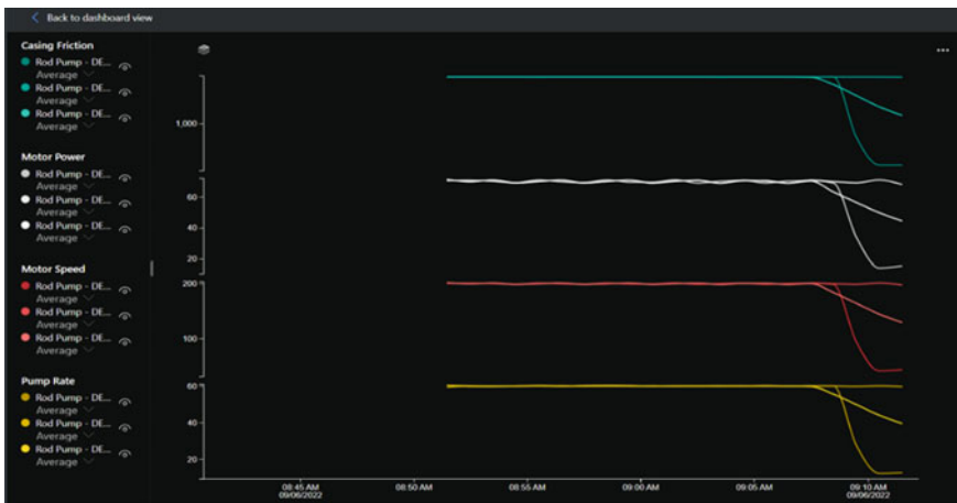
Fig. 14 Dashboard—line chart of casing friction, motor power, motor speed and pump rate for each pump
