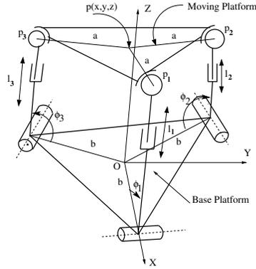
**Fig. 1** The 3-RPS manipulator
