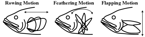
FIGURE 1: TYPES OF PECTORAL FIN MOTION (ADAPTED FROM [24]). THE ROTATION AXES FOR THE ROWING, FEATHERING, AND FLAPPING MOTIONS ARE VERTICAL, TRANSVERSE, AND LONGITUDINAL, RESPECTIVELY.
