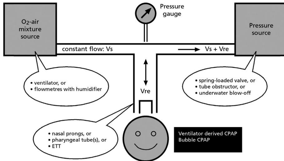
Fig. 3. Continuous-flow positive airway pressure (CPAP) system. ETT, endotracheal tube.
