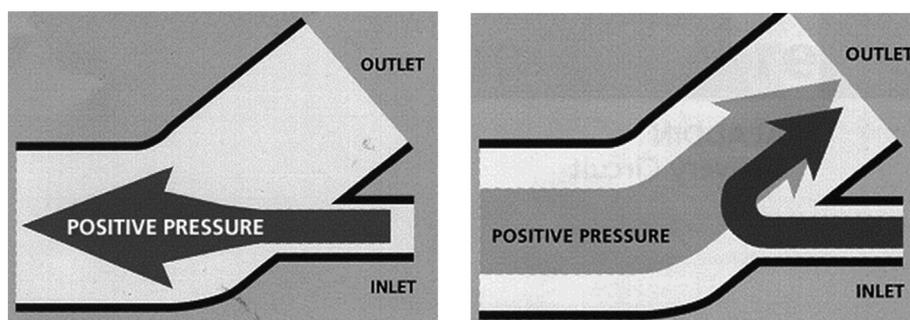
**Fig. 2.** Infant Flow Driver pressure generator. The variable-flow generator uses the Bernoulli principle via injector jets directed toward each naris; Venturi action allows the infant to draw additional gas flow through the injector jets from either the gas supply or exhalation tube reservoir. The dual-jet variable flow generator utilizes fluidic technology to deliver a constant continuous positive airway pressure.
