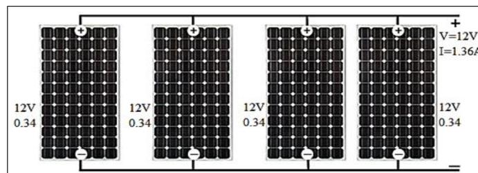
Figure 3. Four PV panels connected in parallel
