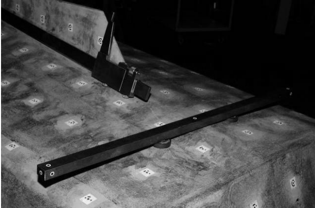
Figure 3: Calibrated steel bar used for scaling.
