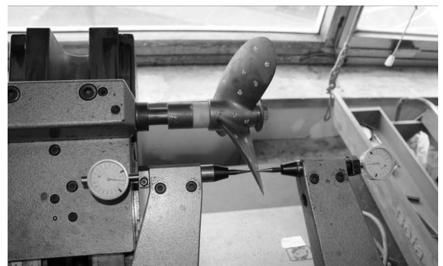
Figure 10: Coordinate Measurement Machine (CMM) specific for screw-propeller models.
