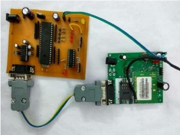
Figure 4: Base station with GSM module
