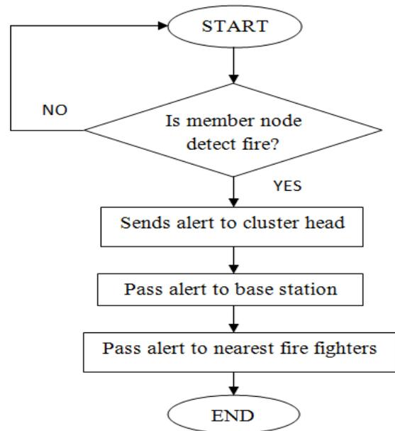
Figure 2: Flowchart for implementation of wireless sensor networks for forest fire detection
