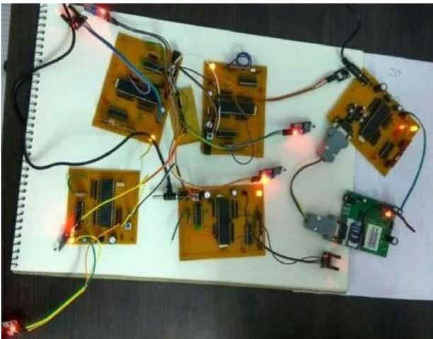
Figure 6: Implementation of wireless sensor network for detecting fire
