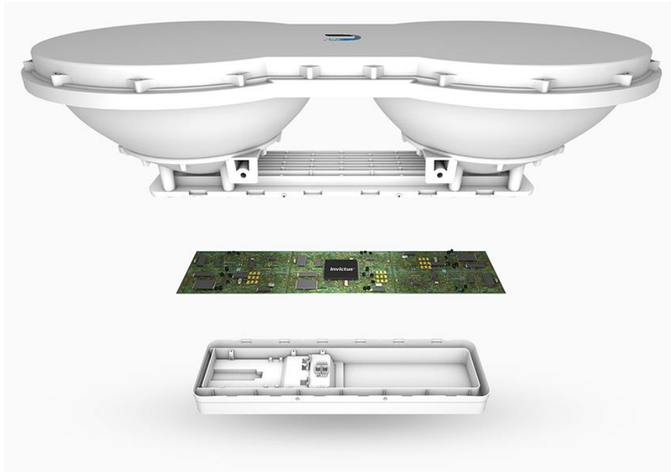
Figure 4. Device and Antenna integration (wifianten, 2016)
