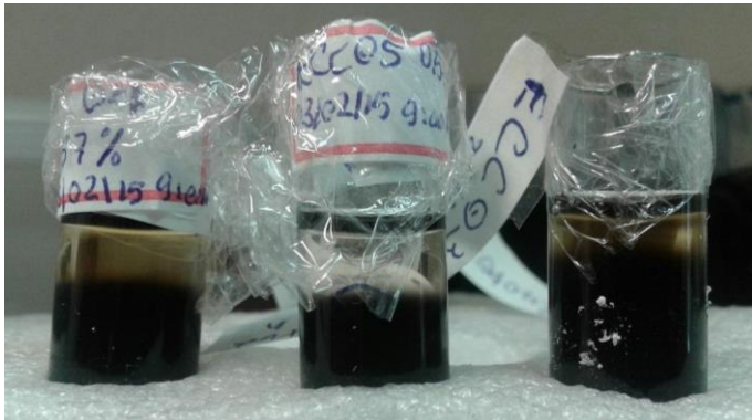
Figure 2. Solubility tests of carbon spherules in glycerol. From left to right, ECC04, ECC05 and ECC03 samples.
