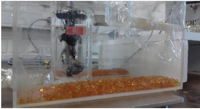
Figure 3. Experimental setup for the dispersion process of carbon spherules in glycerol.
