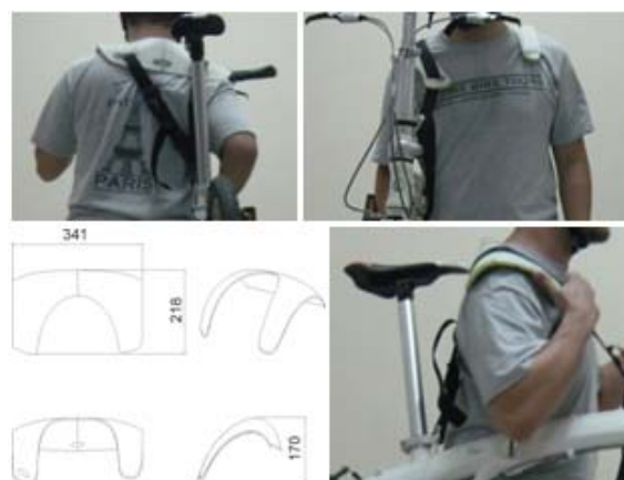
Figure 2 : Dimension and apparatus hooked to the bicycle
