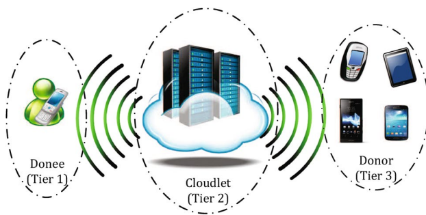
Fig. 1 Computation architecture in Mobile Device Cloud
