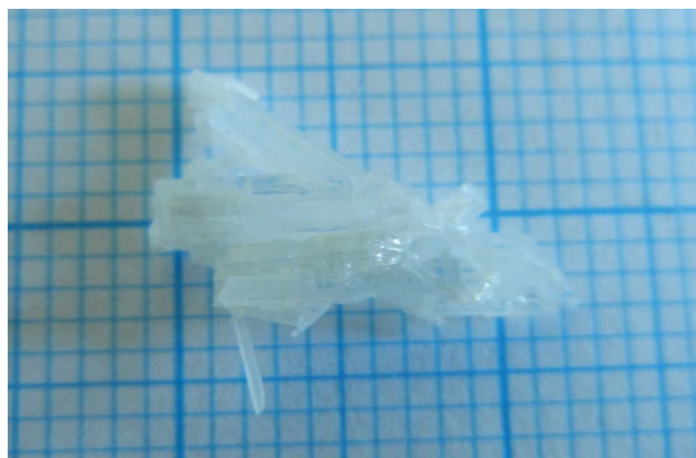
Fig. 4 \text{Ba}_7(\text{BO}_3)_{4-x}\text{F}_{2+3x} crystal aggregate obtained from \text{BaB}_2\text{O}_4 : \text{BaF}_2 : \text{BaO} = 25 : 35 : 45 mol% batch.
