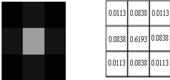
FIGURE 2. DEFAULT FILTER RETURNED BY THE FSPECIAL GAUSSIAN FUNCTION IN MATLAB. SIZE [3 3], SIGMA 0.5
