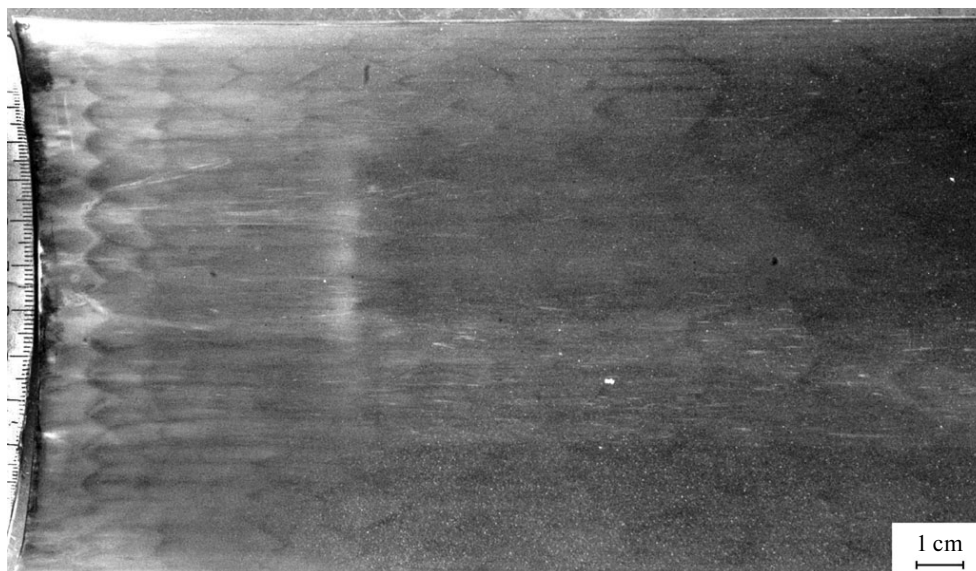
Fig. 3. Soot track of direct detonation initiation for air being present upstream (on the left) of the plate and a \text{H}_2(34\%)+\text{air}(66\%) mixture being present downstream of the plate; the plate is located on the left and is approached by the SW in air from the left.
