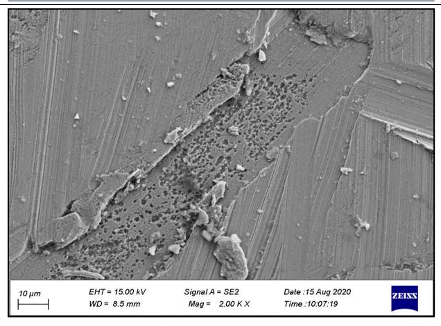
Figure 7: images of mild steel sample in acid medium without inhibitor
