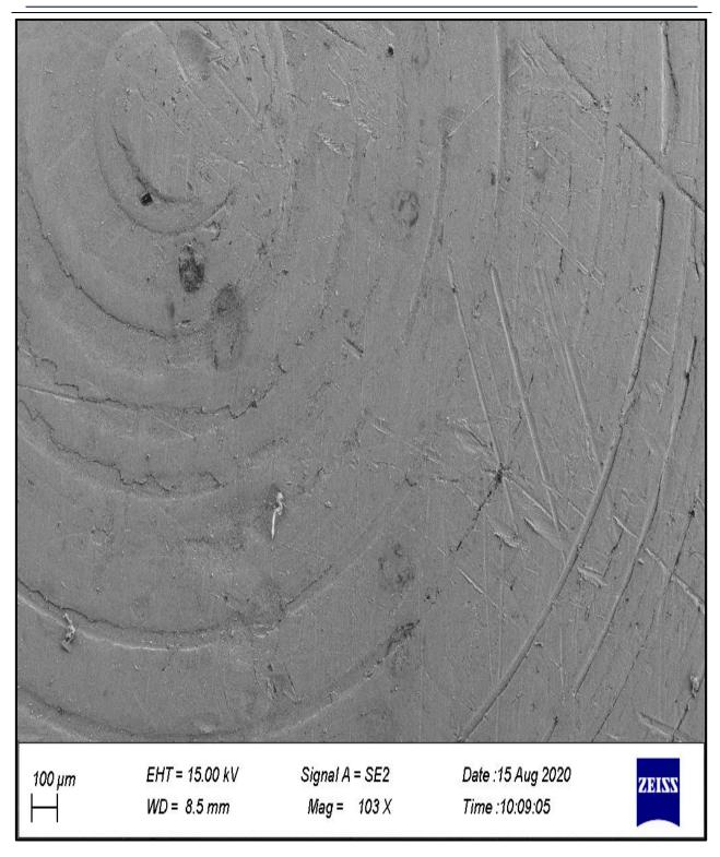
Figure 8: images of mild steel in acid medium witht inhibitor
