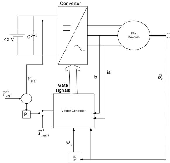
**Fig.6** Block Diagram of ISA system
