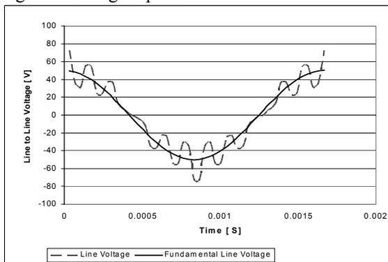
**Fig.3** Magnet induced line to line voltage
