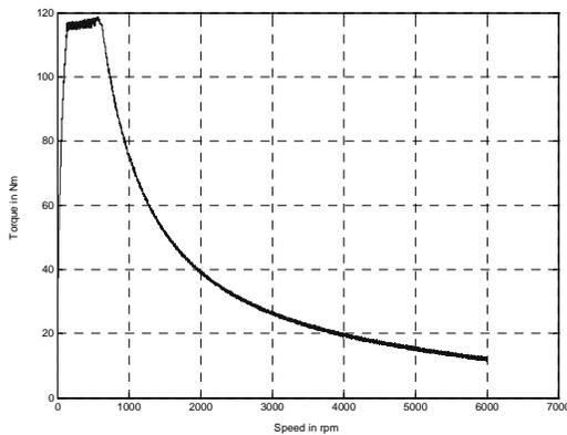
**Fig.7** Torque-Speed Characteristics
