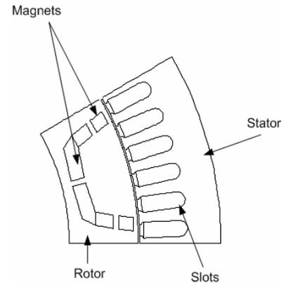
Fig.2 One pole of the machine
