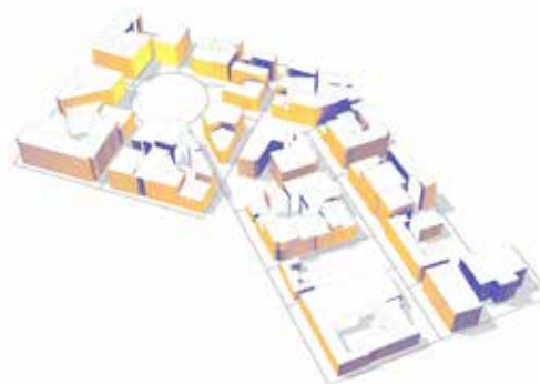
Figure 3 Analysis results (best visible – yellow; non-visible – white), viewing points are distributed along the pedestrian walks with a span of 20 meters.
