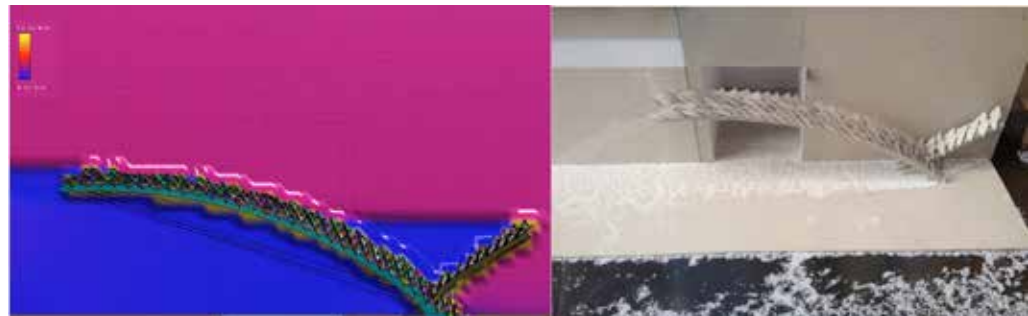
Figure 10 From the left to right: CFD test and wind tunnel test for the final design.
