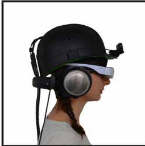
Figure 5 Video glasses and sound system for augmented reality set-up ("Haller interactive")
