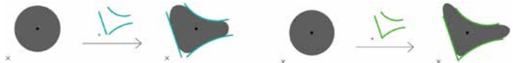
Figure 16 Visual Rule 1 elaborated: Angularity of the plaster object increases as the volume of the outer rigid mold gets smaller.
