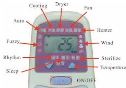
Figure 2 AC controller key functions.
