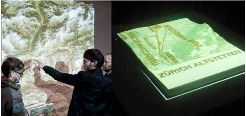
Figure 2 Testing different ways of presenting large scale topographical information by projecting animated informa- tion to a CNC milled model.
