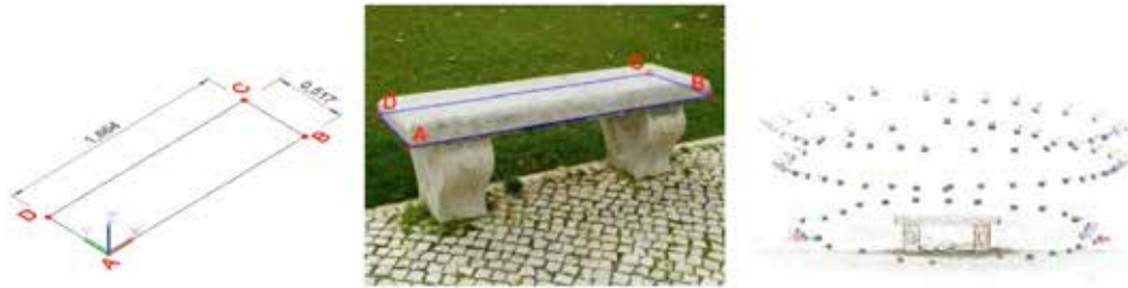
Figure 1 Left: illustration of a reference frame. Center: Cameras relative orientation. Right: Dense point cloud.
