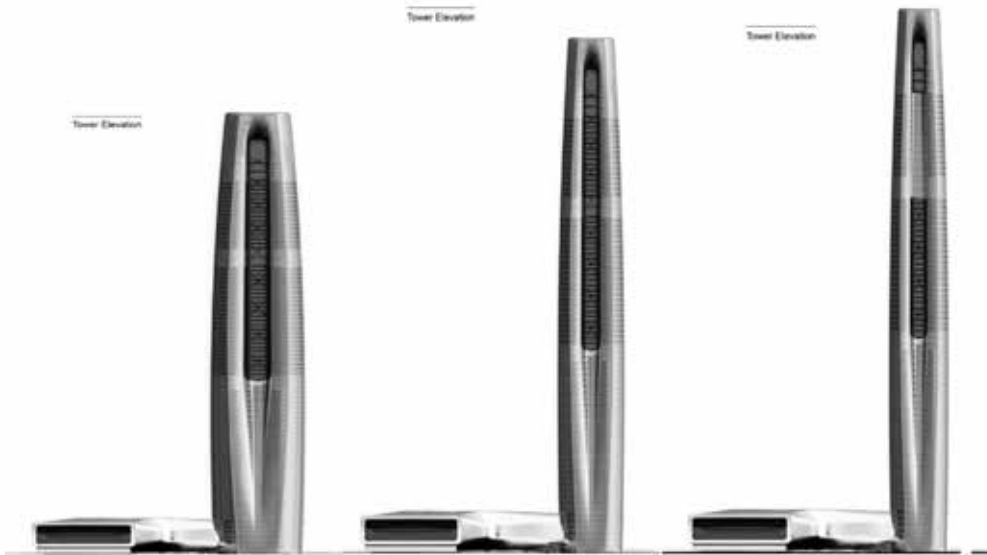
Figure 5 A range of tower designs generated from the student's parametric model.
