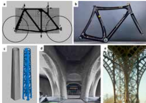
Figure 1 a: Topology optimization method for designing of bicycle [1], b: COLNAGO monocoque bike frame designed using FEA, c: FEA applied in designing of a tower [1], d: Casted free form concrete column by Arata Isozaki in Shanghai, e: Close-up of Eiffel tower column with similar morphology with steel elements.
