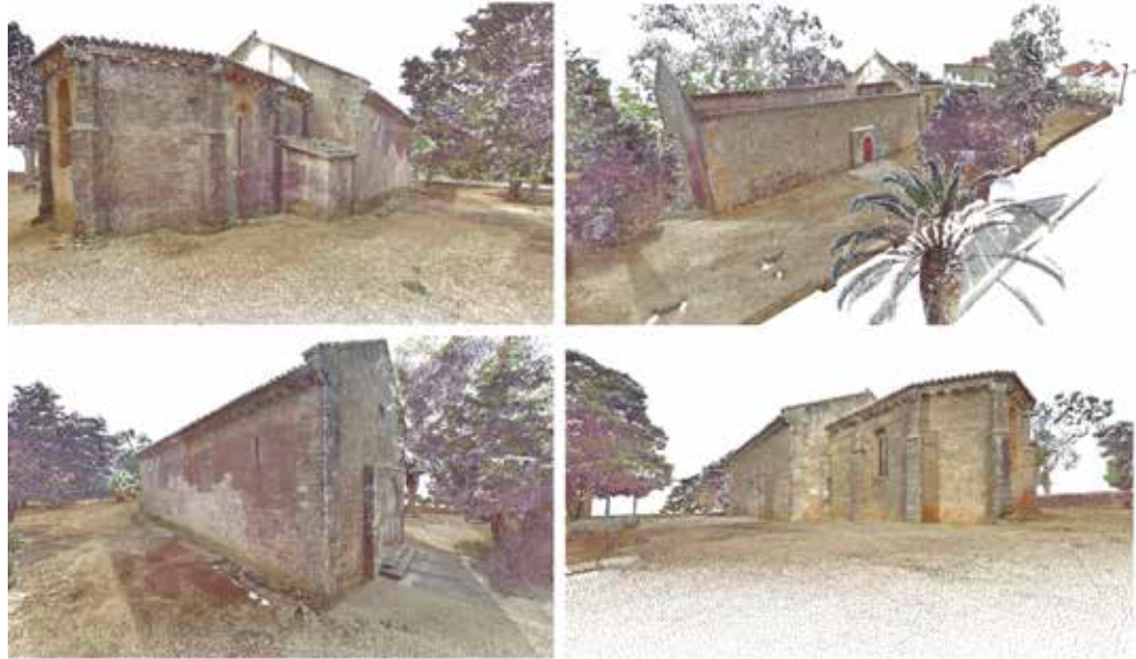
Figure 3 One of the point cloud models that resulted from the second exercise.
