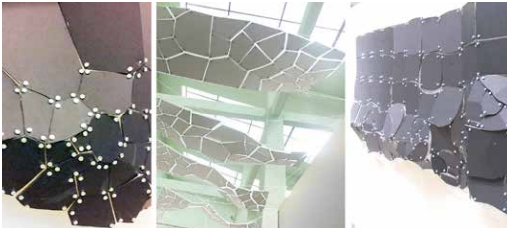
Figure 13 Re_Flex Patterning; Initial prototypes, testing the composite material with various tessellations.
