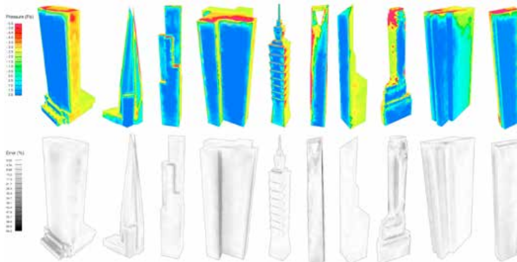
Figure 6 (Upper) Predicted pressure, Pa; (Lower) Error, %. Pressure range is the min. and max. of the entire set for comparison, the error range is absolute max. error of the set (65.2%). (Left to right) (1) Metlife Building, NYC; (2) The Shard, London; (3) Willis Tower (Sears), Chicago; (4) Euston Tower, London; (5) Taipei 101, Taiwan; (6) Shanghai World Financial Centre; (7) Bank of China; (8) Exchange Place, NYC; (9) Frankfurter Buro Centre, Frankfurt; (10) Washington Street, NYC.
