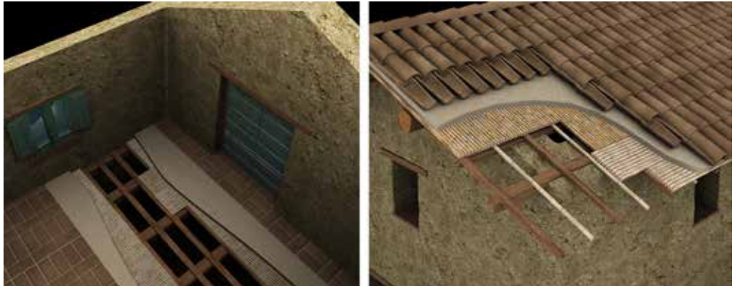
Figure 2 (Left) - the constructive system of the floor (internal view of the room on the first floor); (right) - rendered view of the constructive system of the pitch roof.
