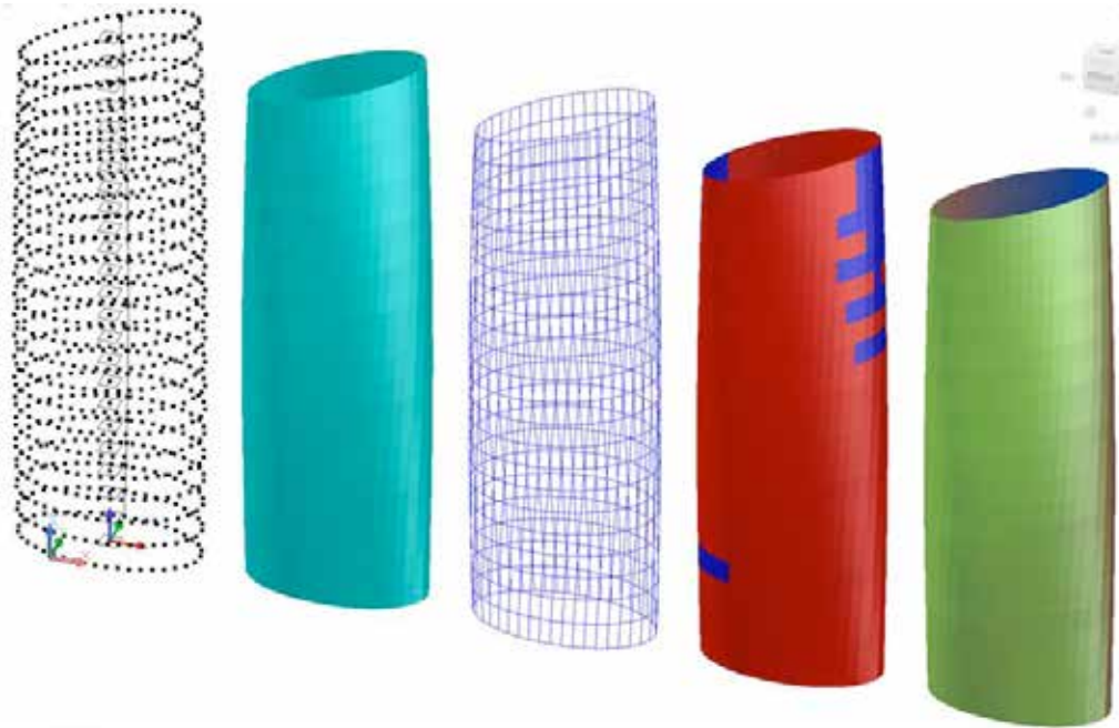
Figure 6 Façade design and analysis with DesignScript, showing the development of a conceptual building model as a series of polygons. Those polygon which are significantly 'out of plane' can be visually identified [indicated in blue in the model, second from the right] and this condition can be used in a downstream fabrication process, for example by switching to different types of facade panels.
