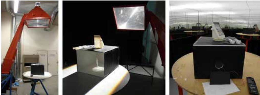
Figure 6 Test settings: From left: Solar Simulator at a 90° altitude (Test 1), Solar Simulator inclined at a 30° altitude (Test 3). Artificial Sky Simulator (Test 4).
