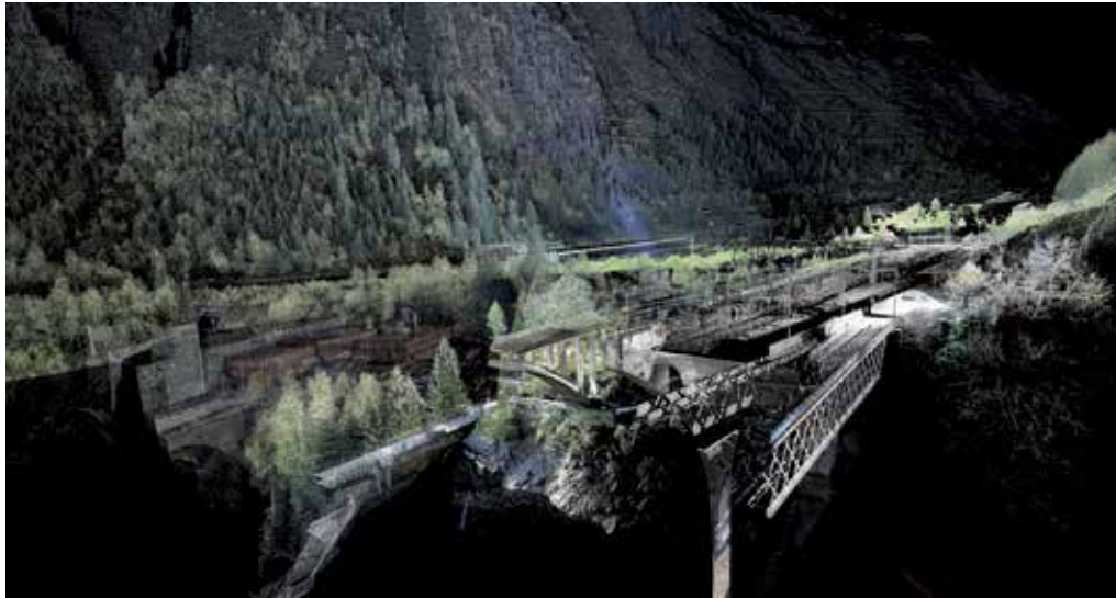
Figure 1 Generated Data: Combination of point cloud data from airborne and terrestrial laser scanner.
