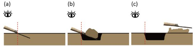
Fig. 4. Three phases of excavation: (a) initialization, (b) ground deformation and clod generation, and (c) clod fragmentation.
