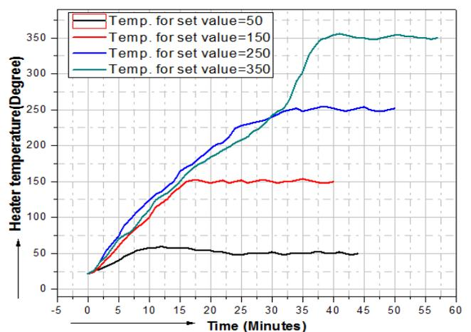
Fig.4. Temperature VS time curve for Set value of  $50^{\circ}\text{C}$ ,  $150^{\circ}\text{C}$ ,  $250^{\circ}\text{C}$  and  $350^{\circ}\text{C}$
