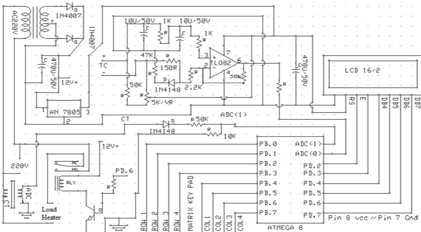
Fig.2. Complete Circuit Diagram
