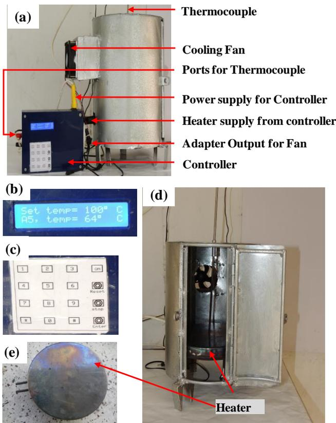
Fig.3. Complete arrangement (a) temperature controller with heater (b) display (c) keypad (d) inner view (e) heater
