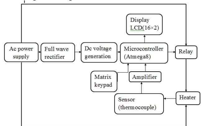
Fig.1. Block diagram of the digital controller
