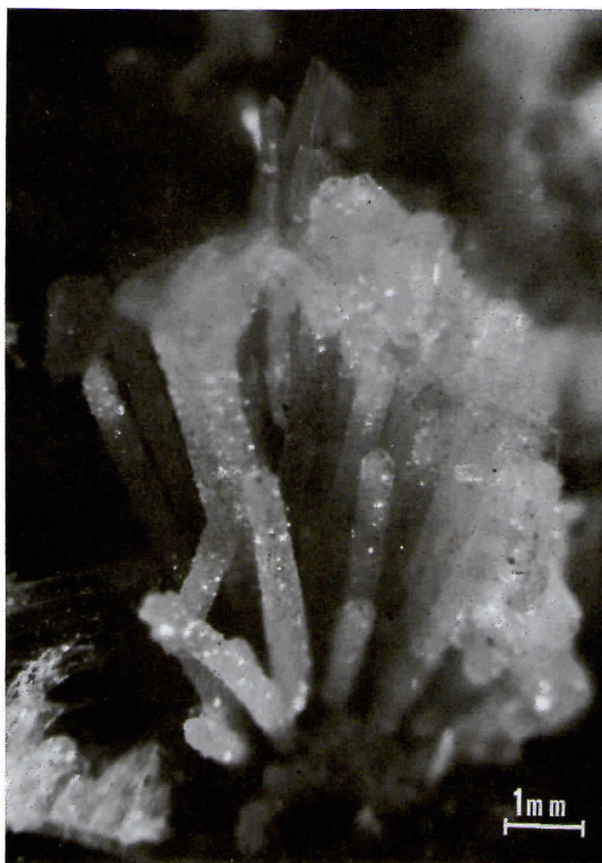
FIG. 2. — Optical micrograph of columnar aggregate of katoite crystals (photo B. Turconi).
