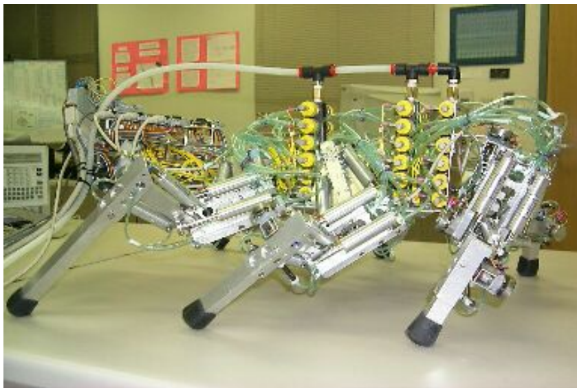
Figure 2 : Protobot [5]. Protobot is modeled after Periplaneta americana cockroach. It has 18 DOF. It uses the double acting cylinder actuator.
