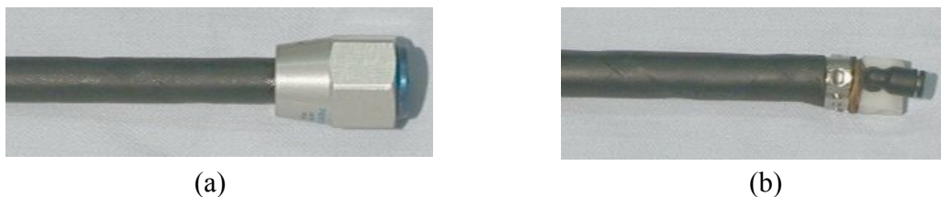
Figure 41 : Festo actuator. (a) original Festo air muscle end. (b) modified end.
