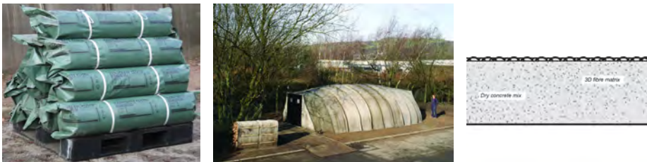
Figure 2.9: Concrete Cloth; left image: sealed rolls; middle image: inflated shelter; right image: build-up of the material (Nuna Innovations Inc. / Concrete Canvas)
