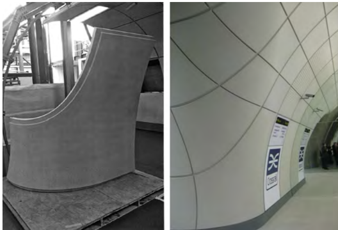
Figure 5.8: Double-curved interior cladding panels in a mock-up for the new Crossrail Line in London (Bull, 2011)
