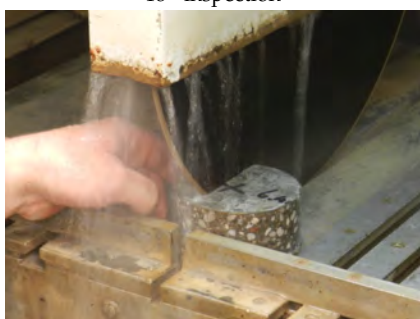
20 - sawing sections for inspection
