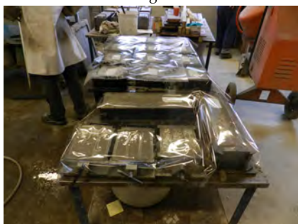
07 - filling and covering cubes and prisms for later testing
