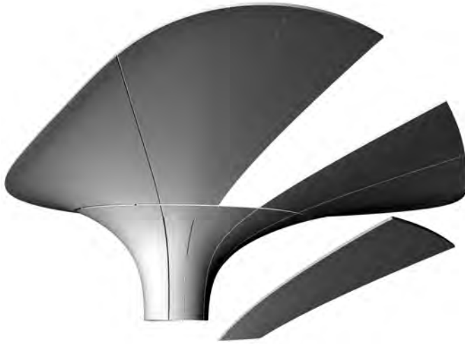
Figure 5.2: Suggested use of thin precast concrete formwork planks for the Spencer Dock Bridge - for an impression of the scale: the element that is shifted from its place has a size of around 1.10 m at the shortest edge, 3.75 m at the opposite edge and a longest edge length of 6.40 m. The thickness in the drawing here was (arbitrarily) chosen as 5 cm. The curvature in two directions is visible.
