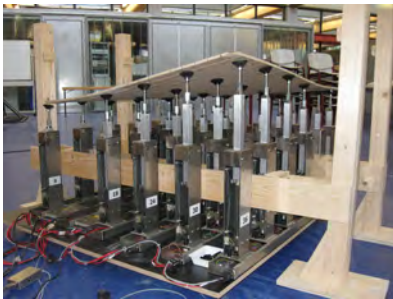
(c) with carved fibreboard surface, left: actuators, right: mock-up panels
