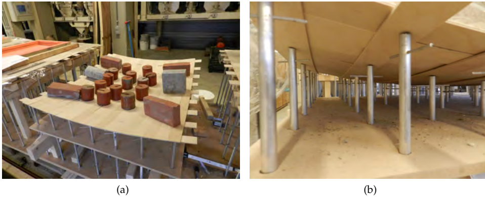
Figure 7.14: Some inaccuracy occurs if strong double-curvature is applied: (a) additional weights are necessary (b) strips not in one plane; small deviations in actuator tips
