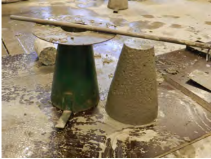
09 - waiting for and testing initial yield strength development
