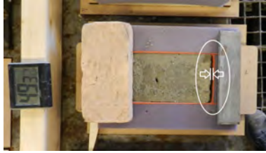
Figure 9.40: Imposed deformation of small specimens - in this case the top surface has elastically shortened, leaving a gap of 2 to 5 mm between mould and specimen
