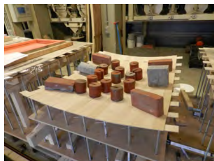
02 - setting up and checking mould shape
