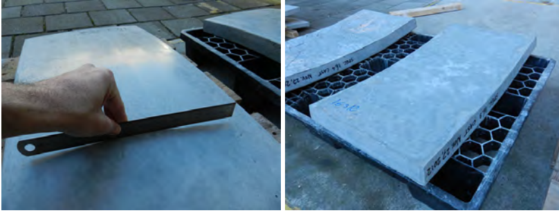
Figure 9.27: Batch 16 - visual inspection of elements; element thickness is 50 mm, radius in two directions is - 2.5 m; the elements are shiny since new silicone moulds were used (PR)
