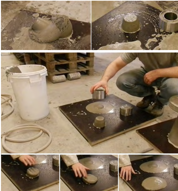
Figure 9.29: Difference between Abrams cone (top-left) and Haegermann cone (top-right) with slump tests at same moment and with same mixture.
