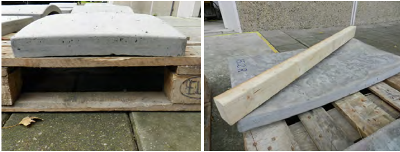
Figure 9.26: Batch 15 - double-curved panel 15.2 with thickness of 50 mm and radius of \pm 2.5 m in two directions
