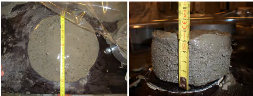
Figure 8.16: Mini-slump tests with PVC-rings for mixture m_1 at t = 1:30 h:min (left) ; mixture m_2 at t = 0:45 h:min (right)
