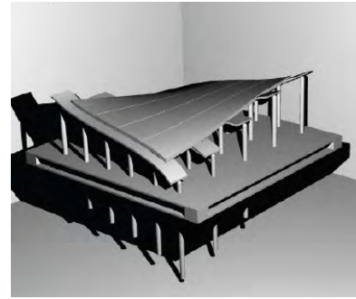
(b) Flexible mould from two layers of strips
