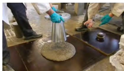
04 - testing slump flow
