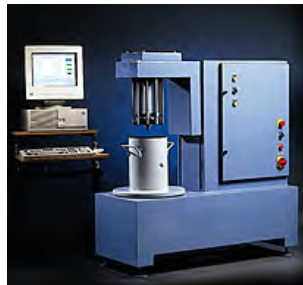
Figure 9.11: ConTec BML Viscometer
