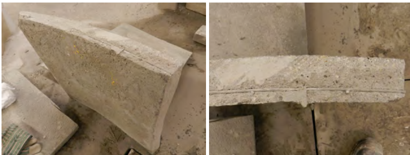
Figure 8.29: Cross-section of the element from test 8 after cutting: the reinforcement has followed the curvature within reasonable accuracy
