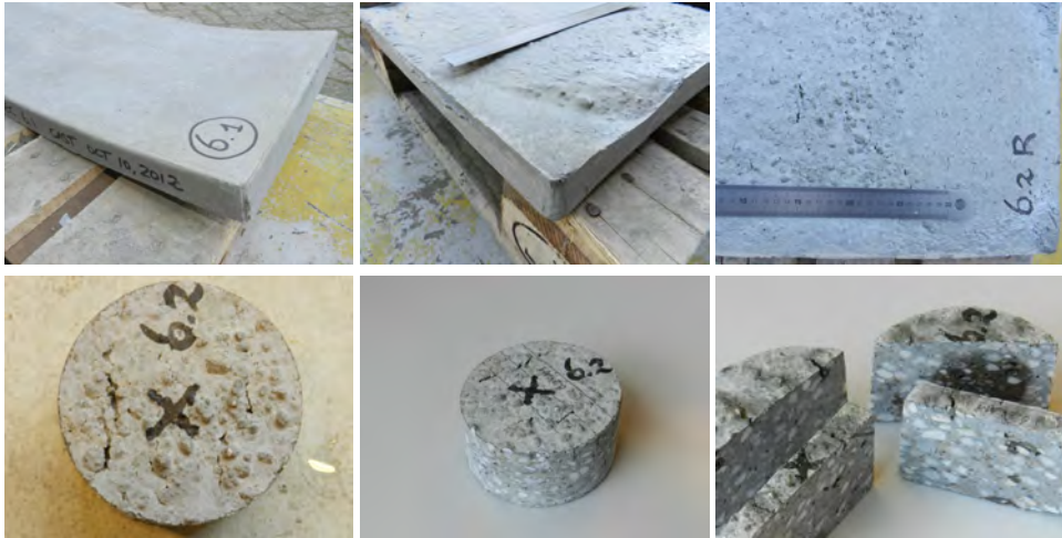
Figure 9.20: Batch 6 - segregation problems lead to bleeding of cement water and unequal element thickness - furthermore cracks appeared in the finishing surface of element 6.1 and 6.2. Cores were drilled and sliced to observe the cracks in more detail
