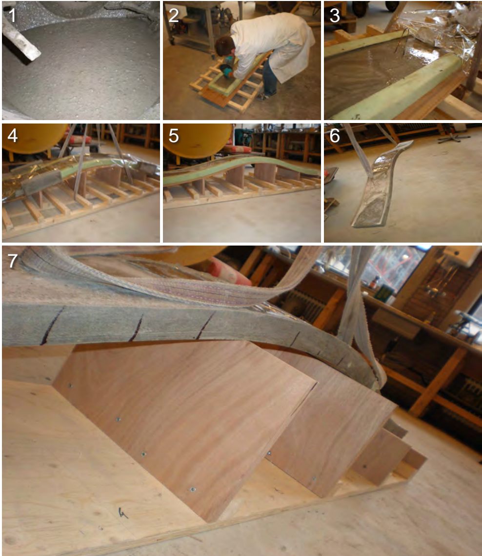
Figure 8.23: Deformation test 5, single-curved element 2.00 \times 0.20 \times 0.05 \text{ m}^3 , \Delta z = 246 \text{ mm} , R_{min} = 1.50 \text{ m} , slope \theta_{max} = 24.6^\circ ; deformation at t = 0:30 \text{ h:min} after casting
