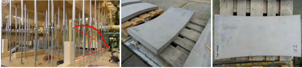
Figure 9.30: Batch 18 - Tilted mould for element 18.2 over around 30^\circ with the horizontal, so that a lower part of the circle-shape is described. This allowed testing of casting under a slope of around 45^\circ at the edge of the mould (normally only 15^\circ with R_1 = -1.5 m, see Table 9.6 on page 189). As can be seen in the right image, the element was cast successfully
