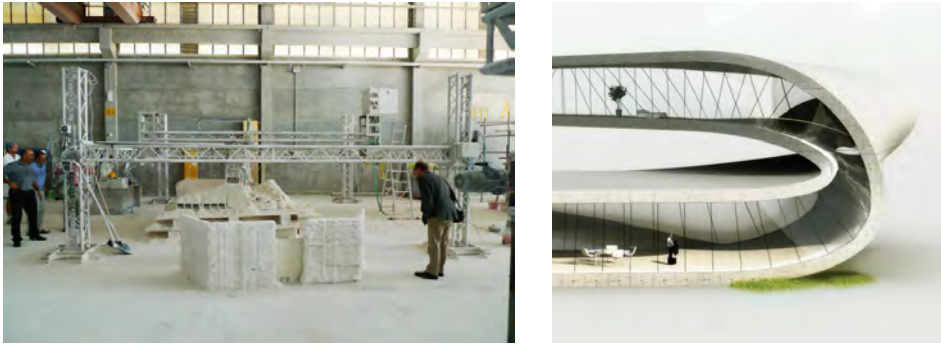
Figure 2.7: left: 3D printer 'D-Shape' using sand and fluid binder of manufacturer Monolite; right: plans for a 3D-printed house with this printer (website ESA / Universe Architecture)
