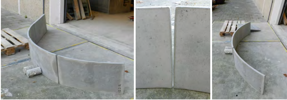
Figure 9.25: Batch 12 - fitting of the cast elements in a curved shape: curvature is quite continuous, edge shape does not fit very well, due to deformation of the mould edge
