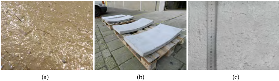
Figure 9.23: Batch 11 - repeated test compared to batch 10 with similar results: cracks in the finishing surface
