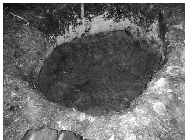
Fig. 9 : Pit constructed near the furnace in which clay is mixed with different additives and kept for 'fermentation'
