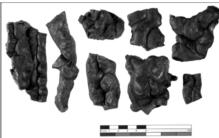
Fig. 5 : Examples of refining slags from Ufipa showing characteristic tap flow morphologies
