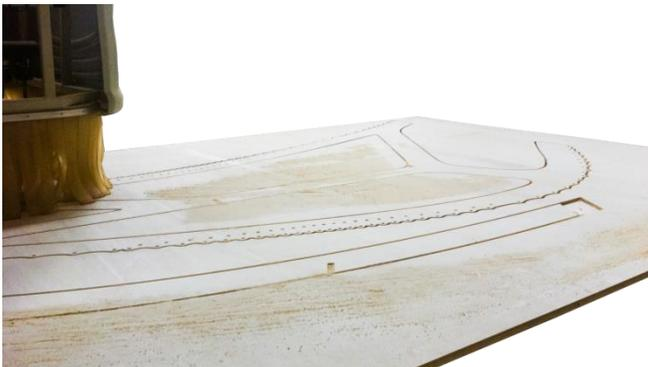
**Figure 12:** CNC milling of a poplar plywood vertical warp and an horizontal support
