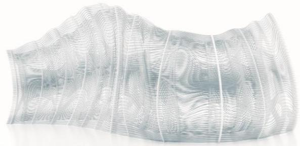
**Figure 15:** Final design configuration of the Weaving Enclosure. The self-standing structure is 7.4 meters long, 3.3 meters in width and reaches a height of 2.9 meters.
