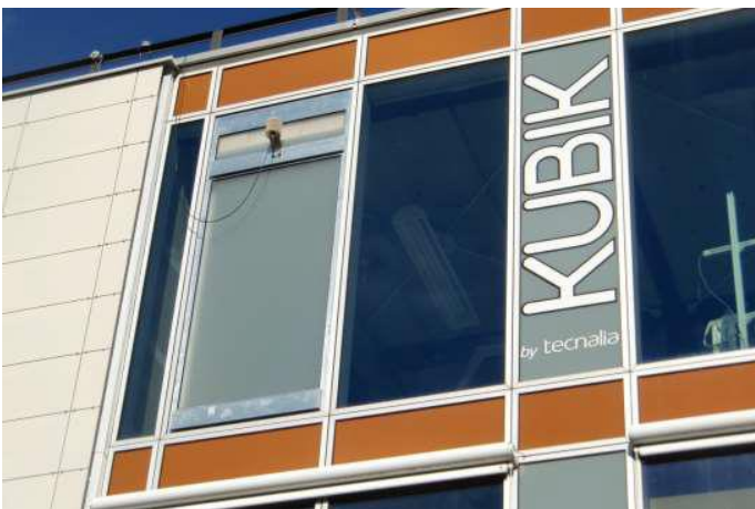
Figure 1: RETROKIT Solar air collector integrated into a curtain wall scheme for testing purposes
