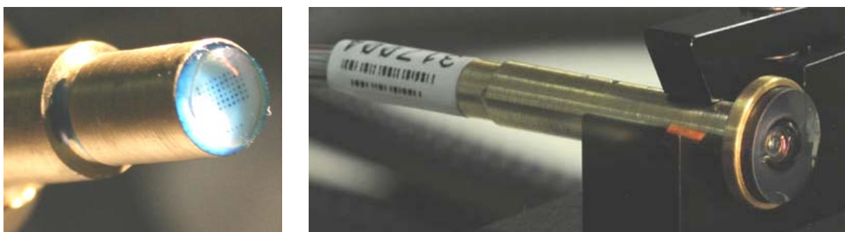
Figure 7. Fisheye probe assembly. Fiber ferrule bonded to index-matching element (left). Assembled unit (right). Photos by Vincent T. Romero and Brian C. Cox.
