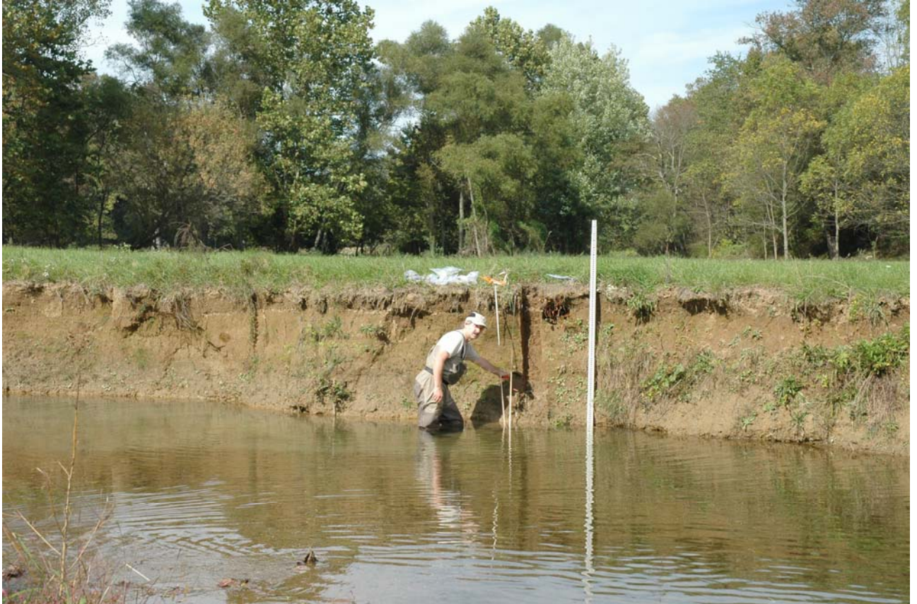
Figure 36. Sampling site for nutrient analysis, right bank E. Br. Codorus Creek, York County. Downstream flow is from right to left. Stadia rod is 3 m in height, and its zero-point is set at the base of the historic legacy sediment (~7 ft thick at this location). A 3 ft layer of coarse, rounded alluvial fan gravel (probably Pleistocene and periglacial) and a thin organic-rich, Holocene pre-settlement layer exist between bedrock and the overlying legacy sediment. Note that the lower part of the legacy sediment is darker. This phenomenon is common, and we interpret it as an indicator that the earliest sediment eroded from the landscape was the organic-rich topsoil. Upper parts of legacy sediment stratigraphic sections along stream banks represent deeper parts of eroded upland soil profiles, and are less organic rich. This reach of the E. Br. of Codorus Creek also was surveyed for bank erosion analysis. We surveyed the bank edge with a high-precision hand-held GPS unit, and compared the bank line to 2003 orthophotography (2 ft ground resolution, +/-5 ft horizontal accuracy). Erosion was not detectable for the three year period, given these image resolution and accuracy limitations. Erosion clearly is occurring at this location, but it must be at a rate that is less than ~10 ft (approximate detectable change) in three years. ARRC (Aquatic Resource Restoration Company) has estimated average bank erosion rates of ~1-2 ft per year.
