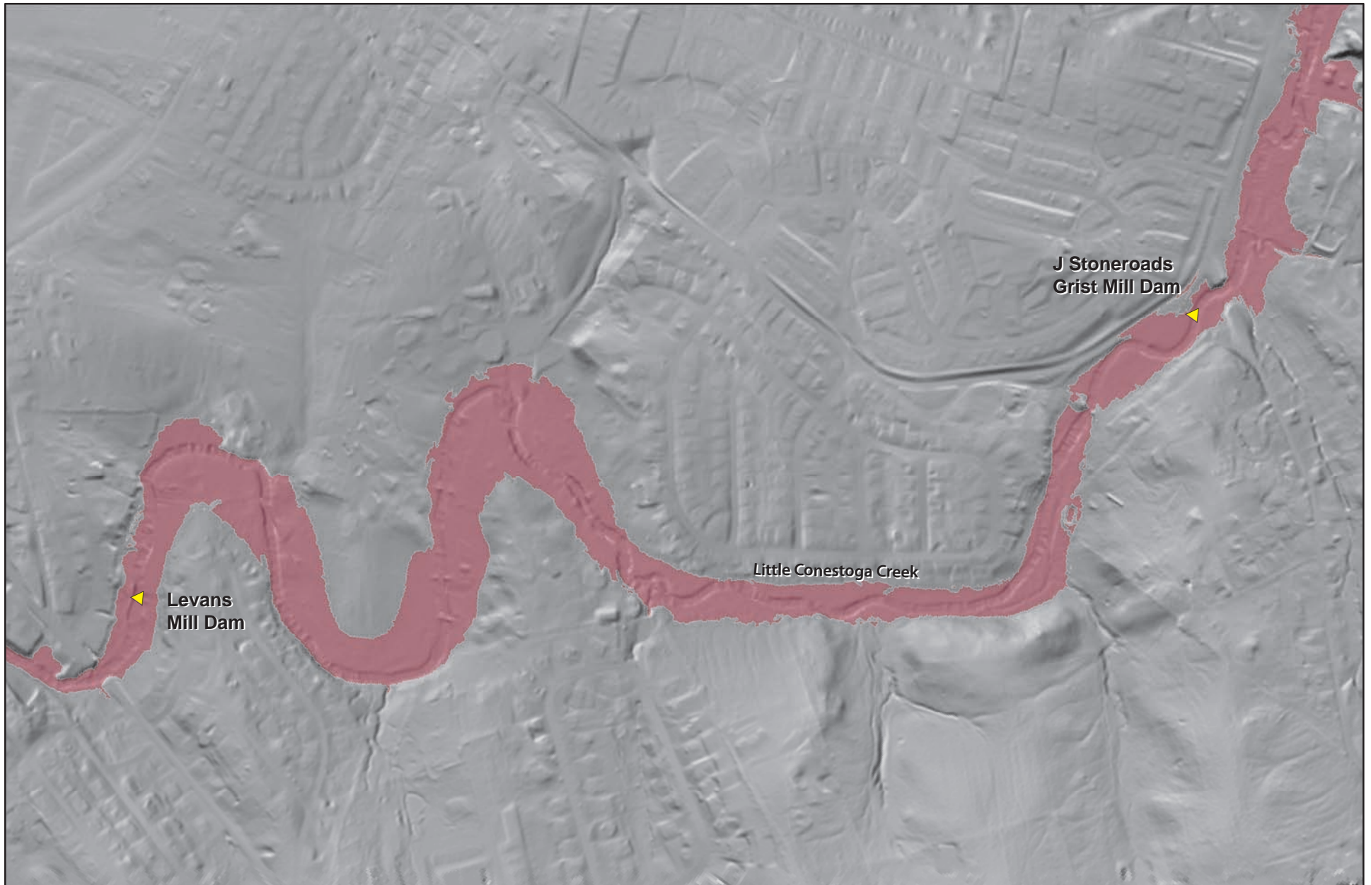
Figure 14 - Legacy sediment extent (red-tinted) above the Levan's Mill dam breach. Direction of flow is from right to left in this view. Legacy sediment forms valley bottom flats and terraces where stream incision has occurred. Hillshade renderings of LiDAR-derived digital terrain models (DTM) clearly depict landscape geomorphology and landscape alteration.
